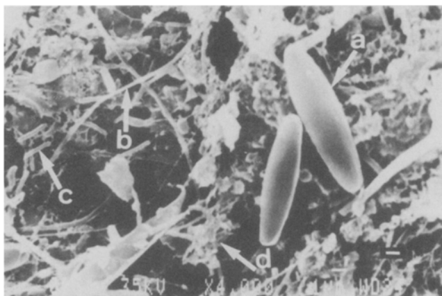
Figure 4 SEM photomicrograph showing biofilm with colonization by algae on stainless steel type AISI-304 coupons after 21 days of in situ exposure to seawater. a, microalgae; b, filaments; c, rod-shaped cells; d, deposits (bar = 1 \mu\text{m} ).
